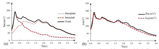
Figure 4. (a)  $Sa(T_1)$  uniform hazard spectra for CU station (interplate and intraslab events) and (b)  $Sa(T_1)$  and  $I_{N_p}$  uniform hazard spectra for CU station.
