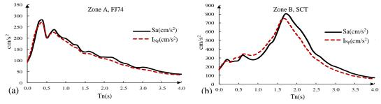
Figure 5. Uniform hazard spectra (250-year return period) for: (a) FJ74 (firm ground) and (b) for SCT (soft soil).
