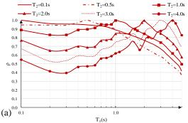
Figure 1. Plots of correlation coefficients versus  $T_1$ , for several  $T_2$  values.
